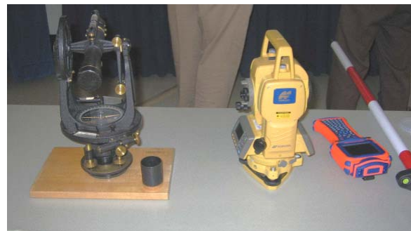
The 'old' optical transit and the 'new' laser transit surveying equipment
