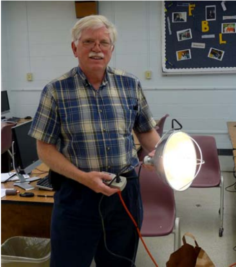
Bill Scott with his 'Kill A Watt' meter proving that a 100-watt equivalent CF lamp does indeed draw only 24 watts.
